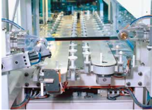
Plexiglas VOD-100 Acrylic Resin material running on DVD line
